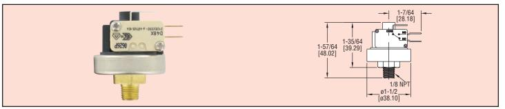
Series A9 Pressure Switches are designed for controlling pressure with higher current capacity. These switches are used widely in steam cleaners, steam irons, and other pressure control systems. It provides SPDT contact and Series A9 Pressure Switches utilize highquality miniature snap-action switches. The switch is diaphragm operated, boasting a high temperature rating and compact size.
